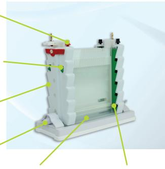
Flat, level gasket prevents current leakage from inner buffer chamber.
