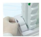
Insert cams and turn until tightened, drawing the PAGE insert onto the casting to form a leak proof seal. **Benefit:** Ultra soft silicone mat within cam-caster to ensure leak free casting.
