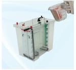
Transfer the PAGE insert to the gel tank. Fill the inner and outer buffer chambers before loading samples.
