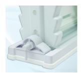
Check the bottom of the glass plates to ensure that they are flush together, and place the PAGE insert on the casting base; make sure that the cams are facing downwards.
