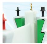
Loosen the vertical screw-pins in the PAGE insert to release the locking mechanism, allowing the gel clamps to sit in the resting slots. 3
